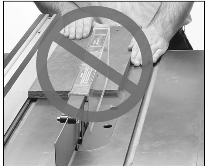
Figure 37. Do not stand directly behind wood.
